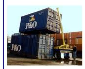
Has the ability to do multiple shifts of containers without having to move the Swing Thru unit
